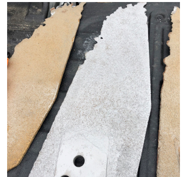
1. Interior of asphalt emulsion tank showing holes from corrosion. Corroded metal mixing blades showing deep pits and missing edges.
